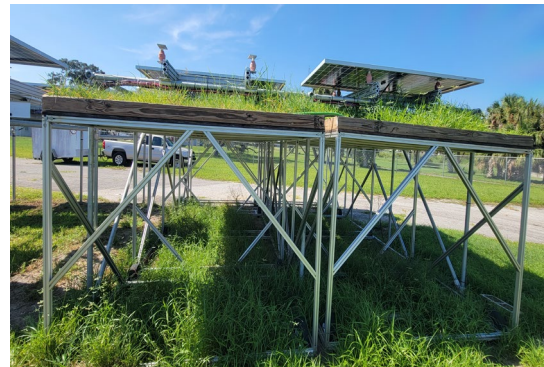
Ground (*1) Modules 30cm above ground
