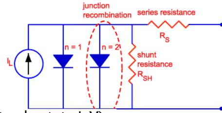
Double Diode Model (DDM) — circuit equation (steady-state I–V)
